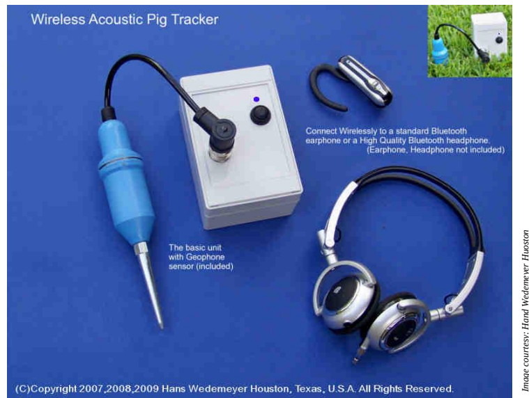
Figure 2-3 : Acoustic tracking using geophones.
