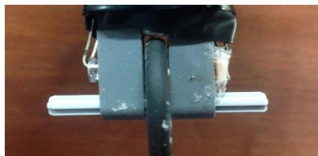
Figure 4-34 : Odometer assembly. Wheel contains LED on one side and a LDR on the other.
